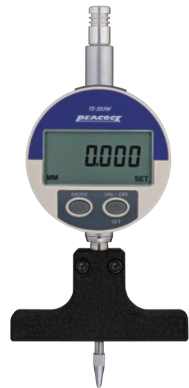
T2-205W Graduation: 0.001mm Range: 20mm
