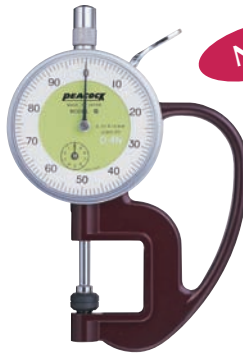
G-0.4N Graduation: 0.01mm Range: 0~10mm
