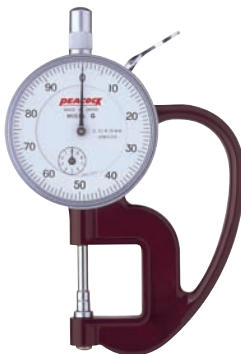
G-1A Graduation: 0.01mm Range: 0~10mm
