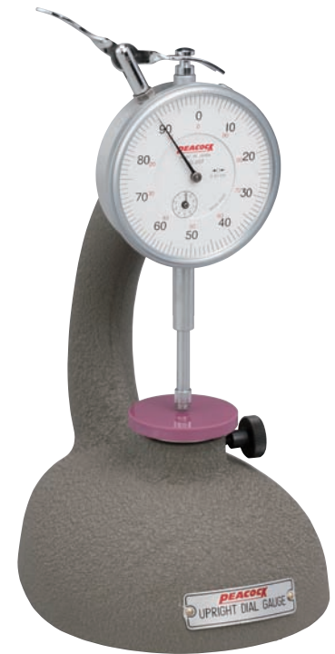
R1-C Graduation: 0.01mm Range: 20mm Effective measuring range: 20mm
