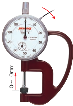
G Graduation: 0.01mm Range: 0~10mm
