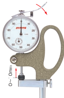
G-3 Graduation: 0.01mm Range: 30mm
