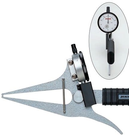
LA-9 Graduation: 0.1mm Range: 0~30mm Throat depth: 100mm
