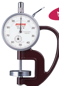
G-30 Graduation: 0.01mm Range: 0~10mm
