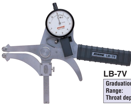
LB-7 Graduation: 0.01mm Range: 10~70mm Throat depth: 85mm ● Adjustable frame
