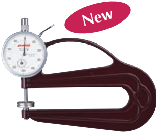
H Graduation: 0.01mm Range: 0~10mm
