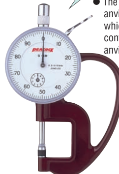
G-1M Graduation: 0.01mm Range: 0~10mm
