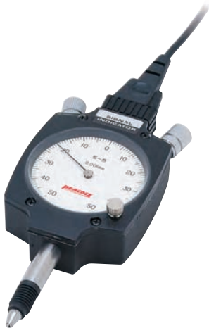
S-5 Graduation: 0.001mm Measurement range: 0.1(±0.05)mm
